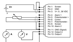
Please use shielded cables for the connection of the device. Strong electromagnetic sources, like power lines close to the converter or its lines should be avoided.
